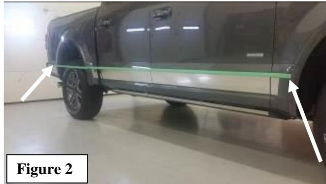
5. Each panel will be numbered 1D/P - 5D/P (for Regular Cab) or 1D/P - 6D/P (For SuperCab and SuperCrew). (D = Driver Side, P = Passenger Side) Determine and verify the exact location for each panel by holding them up to the vehicle, lining the top edge of the panel with the bottom edge of the tape line. Panel #1 should be located behind the front wheel. Panel #2 located on the front door and so on until you reach the last panel located on the bed behind the rear wheel.
