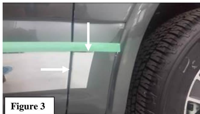
7. Remove and fold down about 1/2" of the red protective film from the entire top side of panel #2. Hold the ends of the panel as you align it to the tape on the front door. When the part is aligned to the door and the tape line, gently press the exposed adhesive part onto the vehicle, while maintaining alignment. Slowly pull the remaining red protective film downward until the film has been completely removed. Press the panel firmly onto the vehicle for 30 seconds to ensure proper adhesion.
