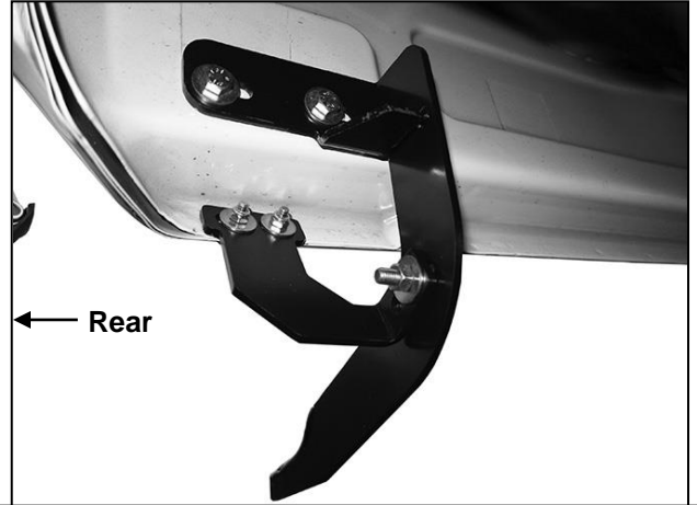
(Fig 18) Driver/Left rear Mounting Bracket assembly
