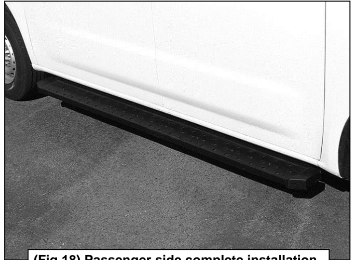
(Fig 18) Passenger side complete installation
