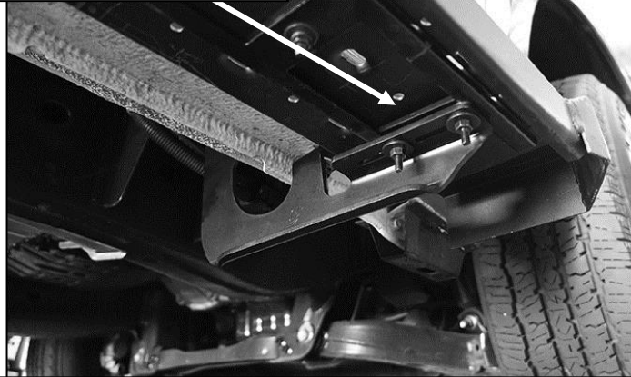
(Fig 17) Passenger front Bracket with Running Board
