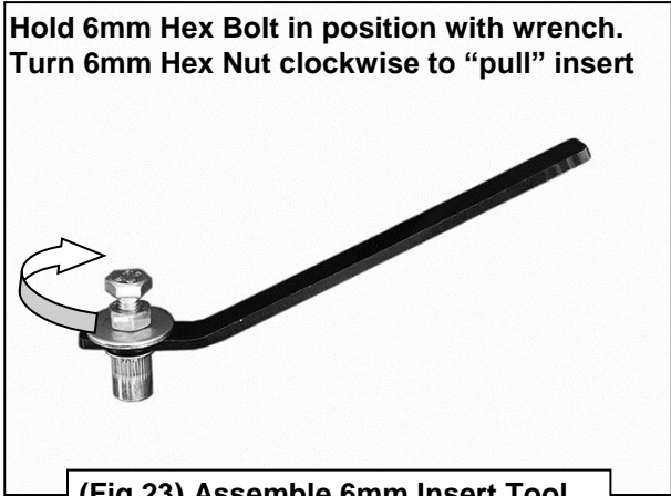
(Fig 23) Assemble 6mm Insert Tool
