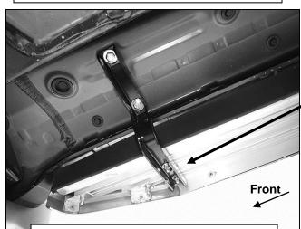
(Fig 8) Front Bracket installation pictured
