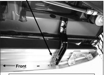
(Fig 9) Rear Bracket installation pictured
