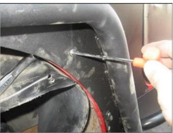
Step 2. Insert bolts through flare and jeep body and hand tighten with lock nuts. (You may need to pull inner fender liner down to gain access to the back of the bolts to install the nuts)
