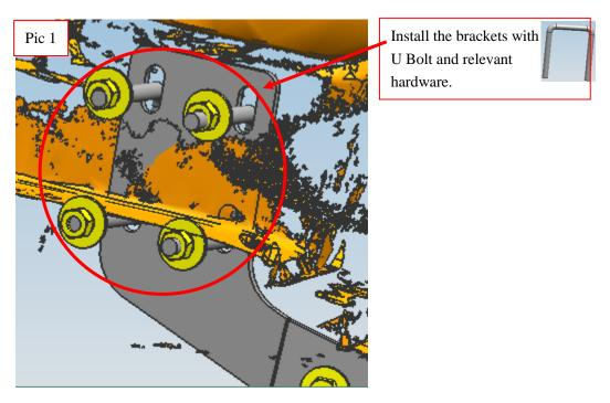
Step 3: Install the side bar on the brackets and tighten up hardware after adjusting the brackets.
