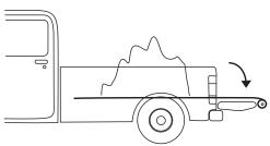
Open tailgate and spray lubricate the Bearings.
