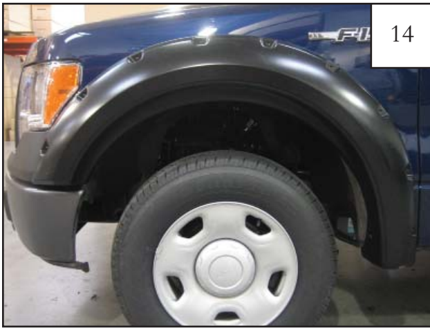
Completed front flare installation.
