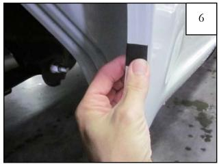
Wrap a Foam Tab (MT1-0034) around the wheel well sheet metal, centered over each of the upper four marks made in Step 15. Place a Mylar Tab (MT1-0014) at the mark made on the lower front of the wheel well.
