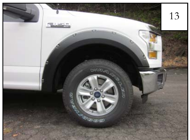
Completed front flare installation.
