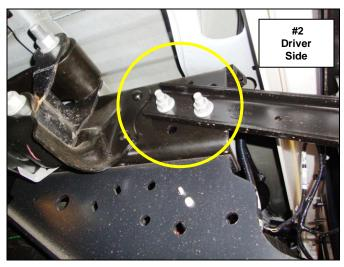
**Step-4** The factory receiver hitch is attached to the bottom of each frame rail with (2) sets of nuts and bolt plates, 2 at the front and (2) at the rear. Remove the nuts and bolt plates at the rear using a 24mm socket and ratchet, (Photo 3). Retain the nuts and bolt plates to install the bumper replacement brackets and reinstall the factory receiver hitch.
