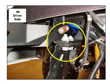
Step-9 With assistance attach the bumper shell brackets to each frame bracket using (2) 1/2" x 1 1/2" hex bolts, (4) 1/2" flat washers, (2) ½" lock washers and (2) ½" Hex nuts, (Photo 7). Align the bumper shell with the vehicle, verify that the tailgate clears when lowered, then tighten the nuts and bolt plate securing the frame bracket to the side of the frame first then tighten all remaining factory and supplied nuts and bolts.
