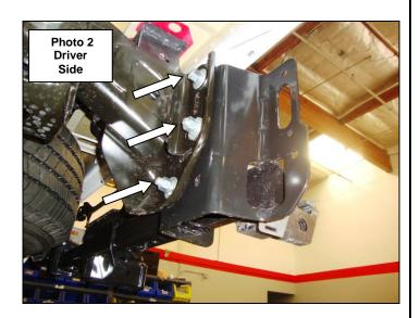
**Step-**9 With assistance attach the bumper shell brackets to each frame bracket using (2)  $\frac{1}{2}$ " x 1  $\frac{1}{2}$ " hex bolts, (4)  $\frac{1}{2}$ " flat washers, (2)  $\frac{1}{2}$ " lock washers and (2)  $\frac{1}{2}$ " Hex nuts, (Photo 3 & 4).
