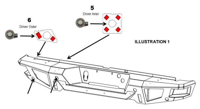
**Step-5** Prepare the inside surface of the bumper shell where the bezel plates will be mounted with Isopropyl alcohol. A clean, dry surface is required in order for tape to stick properly.
