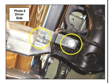
**Step-10** With assistance attach the bumper shell brackets to each frame bracket using (2) ½" x 1 ½" hex bolts, (4) ½" flat washers, (2) ½" lock washers and (2) ½" Hex nuts, Align the bumper shell with the vehicle, verify that the tailgate clears when lowered, and tighten all nuts and bolts, (Photo 7). If necessary loosen the frame / receiver hitch bolts to adjust the bumper shell.
