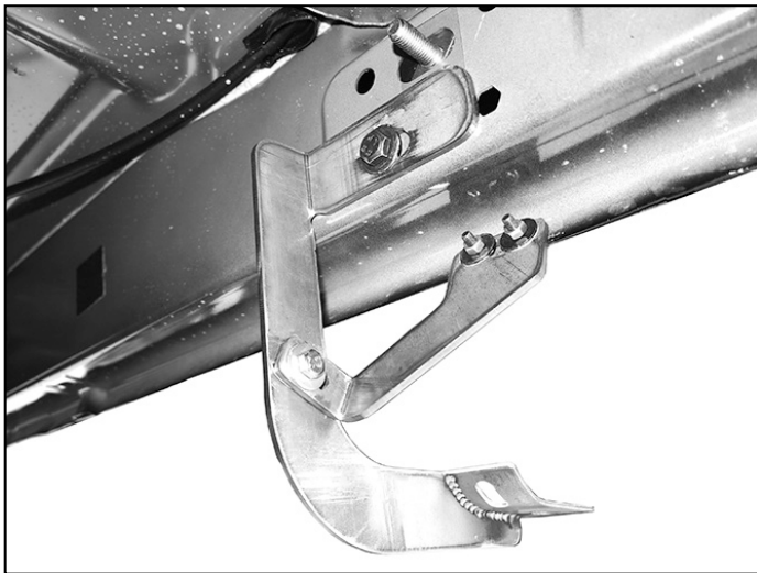
(Fig 7) Driver side 2011-on model with factory holes in pinch weld pictured.
