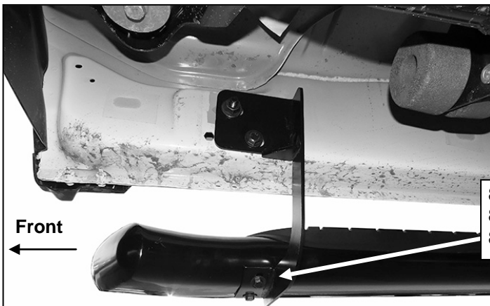
(Fig 15) Passenger/right front Bracket installed
