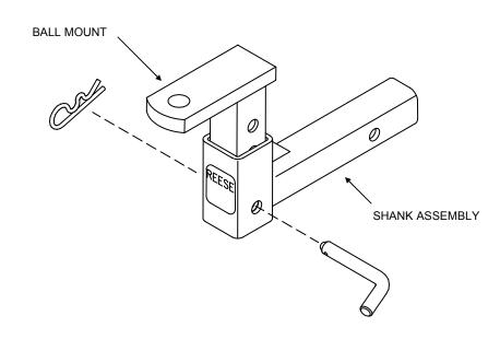
HITCH BALL SELECTION - Ball diameter must match trailer coupler size. The three most common sizes are 1-7/8", 2", and 2-5/16". Select ball with 1" threaded shank that is V-5 rated equal to or greater than trailer gross vehicle weight rating (GVWR).
