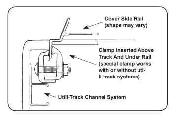
3. Clamping Rail: Loosen nut on clamp enough to allow clamp assembly to insert above Utili-Track system at each end. Then slide clamps into position along length of box. Use all clamps in kit—half on each rail. For all remaining clamp and rail installation, see Owner's Manual. Finish in stalling both side rails now.
