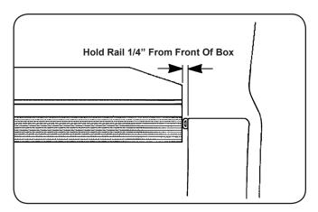
2. Aligning Front of Side Rail: Front of rail should be set 1/4" away from front of box.
