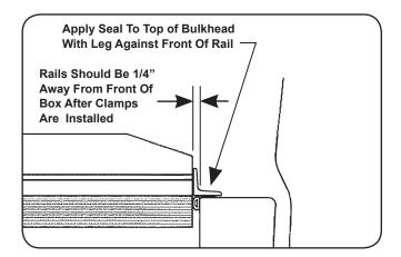
4. Element Seal Option: Certain model covers come standard with front Element Seal. Install this seal to top of bulkhead from side to side as shown. OMIT THIS STEP FOR COVERS WITHOUT THIS SEAL. Follow Owner's Manual for remaining cover installation.
