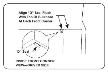
Installing "D" Seal: Clean surface where seal adheres. Peel off backing. Adhere seal flush with top of bulkhead on inside of front corner as shown. Repeat on opposite front corner.
