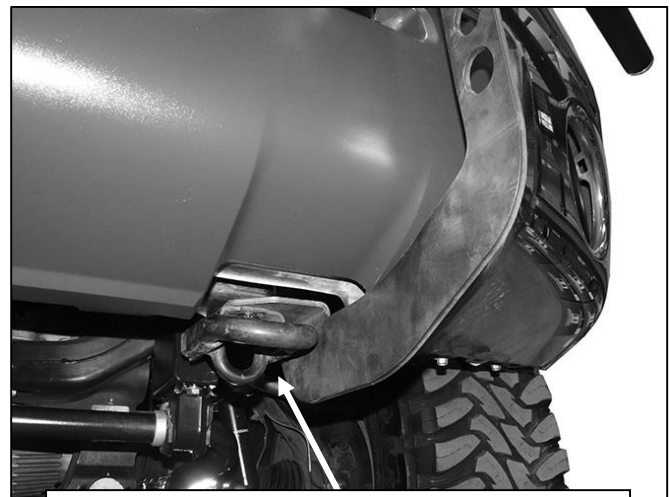
(Fig 14) Line up the Lower Frame Bracket between the tow hook mounting location and the tow hook. Use the factory bolts to reinstall the tow hook over the Bracket
