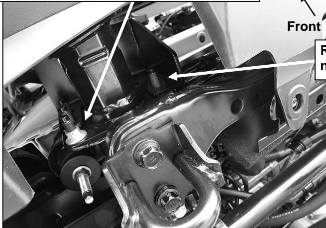
(Fig 6) Passenger side Upper Frame Bracket installed over bumper bracket. Pictured from below
