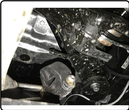
2. Fishwire (2) 7/16" carriage bolts and (2) CM-SP2 spacers through the vehicle access holes to the attachment holes on each side.
