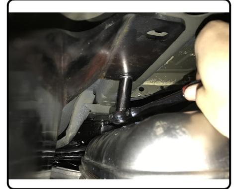
6. Secure Tow Loop Plate to recovery loop using (1) 1/2" bolt, (1) CM-SP32 spacer and (1) 1/2" hex flange nut. Torque all 7/16" hardware to 59 ft-lbs and all 1/2" hardware to 110 ft-lbs. Reinstall Hands Free Access sensor if removed in Step 3. To raise exhaust follow Step 1 in reverse order.
