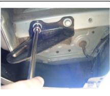
2) Lower rear most exhaust isolator for ease of installation.
