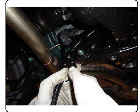
2. Remove (4) heat shield attachments with phillips head screwdriver or 10mm socket (both sides if equipped with dual exhaust). Remove three hole plugs from each side of frame to expose mounting holes. Return all removed items to customer.
