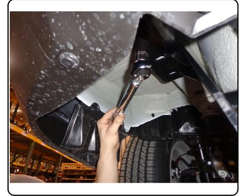
6. Raise exhaust back into place and reattach exhaust hangers. Install complete.
