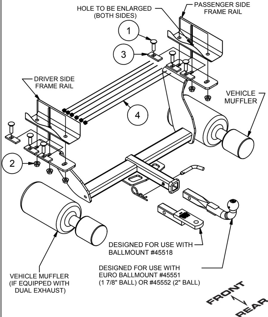
1. Remove (2) exhaust hangers from the passenger side muffler and (1) exhaust hanger from the center front of vehicle for single exhaust vehicles, dual exhaust will remove (2) exhaust hangers from the driver side muffler as well. Support lowered exhaust with jack stand.
