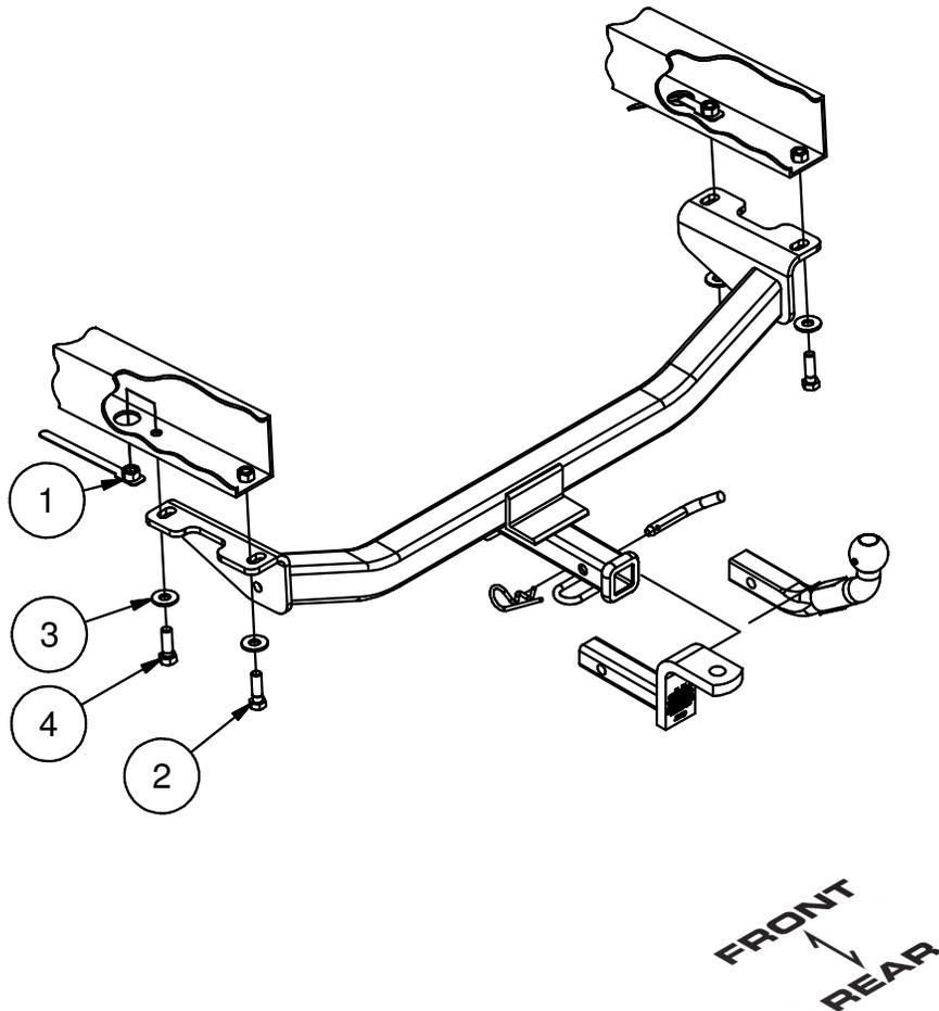
1. Locate (2) existing weldnuts in rear of vehicle frame. Spray lubricant or compressed air into hole. For heavy debris, use a small wire brush. (Be careful not to damage threads.)
