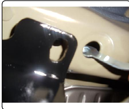
4. Use 1/2-13 hex bolts and 1/2" conical toothed washers and insert hardware through hitch plate and vehicle frame into the handle nut and tighten.
