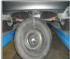
2. Fishwire 1/2" carriage bolts and CM-SP12 spacers into vehicle bumper beam.
