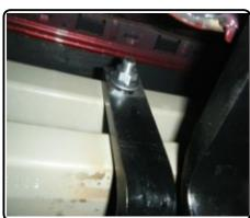
4. Fishwire 1/2" carriage bolts and CM-SP6 spacers into vehicle "A" frame and secure with 1/2" hex flange nuts.
