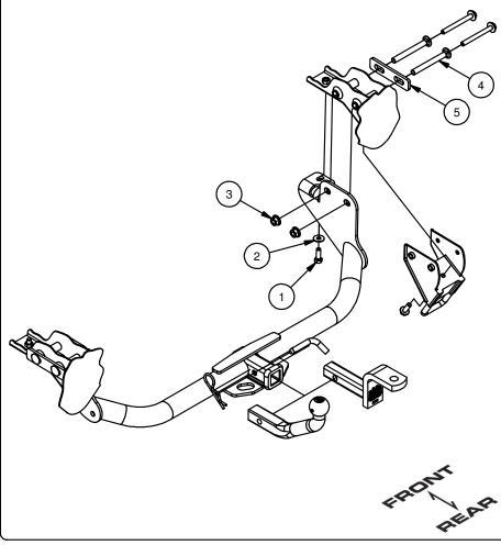
1. Remove (3) bolts and tow loop from the passenger side frame rail. Return bolts and tow loop to owner
