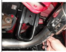
2. Insert 1/2-13 x 4 1/2" carriage bolts and CM-12048-SP spacers through the existing holes in the side of the frame rails. After bolts are inserted push them back so the end is flush with the inside of the frame rails.
