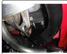
4. Align the bottom tabs of the hitch with the weldnuts in the frame rails and secure with M10-1.25 x 25mm bolts and 3/8" conical toothed washers.
