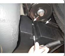
2. Locate (2) weldnuts near the end of each frame rail. Clean weldnuts of debris and rust to ease hitch installation.
