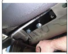
4. On the driver side frame rail fishwire a 7/16-14 x 1 1/2" carriage bolt and CM-SP2 spacer through the access hole and into the existing hole in the bottom of the frame rail. Secure with 7/16" flange nut.
