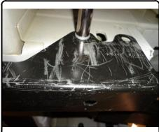
3. Fishwire (1) 1/2 bolts and spacers into each bumper frame rail.
