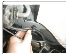
4. Lower exhaust by removing two to four (depending on vehicle) rearmost rubber hangers. Leave rubber hangers attached to the vehicle.
