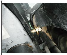
9. Pull 1/2" hardware into position & remove fishwire(s). Fasten with 1/2" hex flange nut(s). Re-secure harness which was unfastened in step 3. Wrap cable tie(s) around hitch mounting plate(s) and harness. Pull tight & trim excess cable tie.
