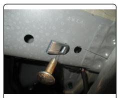
4. Gently pull fascia down and raise hitch into position guiding fishwires through mounting holes. NOTE: Hardware may need to be temporarily pushed into frame to position hitch over bumper beam studs. Remove fishwires & loosely secure 7/16 nuts. Secure existing M10 nuts onto bumper beam studs.
