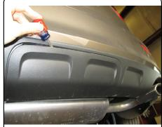
2. Remove (2) screws holding bumper fascia using a T15 torxbit. Save screws for re-installation. Use a 15mm deep well socket to remove (1) M10 flange nut from the bottom of driver side bumper beam attachment location & repeat on passenger side. Save nuts for re-installation.
