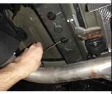
2. Raise hitch into position securing with supplied M12 bolts and conical washers. Torque all hardware to 86 ft-lbs.
