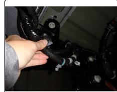
4.) Using the existing mounting hardware, attach the bottom mounting bolts (2 places each side) and loosely secure so that bumper placement adjustments can be made. Adjust bumper position to align with side mounting holes and secure remaining (4) bolts with a 21mm socket.
