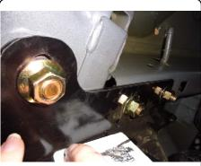
6.) Raise exhaust back into position and reinstall the (6) rubber isolators removed in Step 1.
