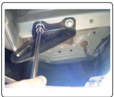
2. Lower rear most exhaust isolator for ease of installment.
