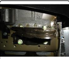
2. Lower spare tire using tire lug wrench or ratchet with 21mm socket.
