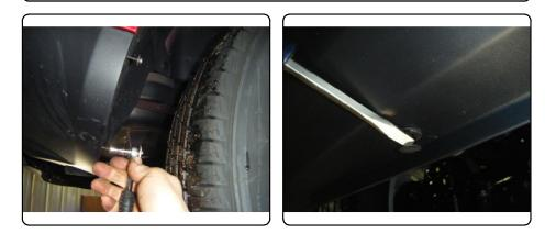
Lower exhaust by removing (3) rubber isolators. See RUBBER ISOLATOR REMOVAL DIAGRAM on page 2.
