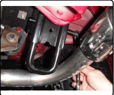
Insert 1/2-13 x 4 1/2" carriage bolts and CM-12048-SP spacers through the existing holes in the side of the frame rails. After bolts are inserted push them back so the end is flush with the inside of the frame rails. <u>Note</u>: On the driver side, reach between the bumper cover and rear wheel well to access the holes in the side of the frame rail.
