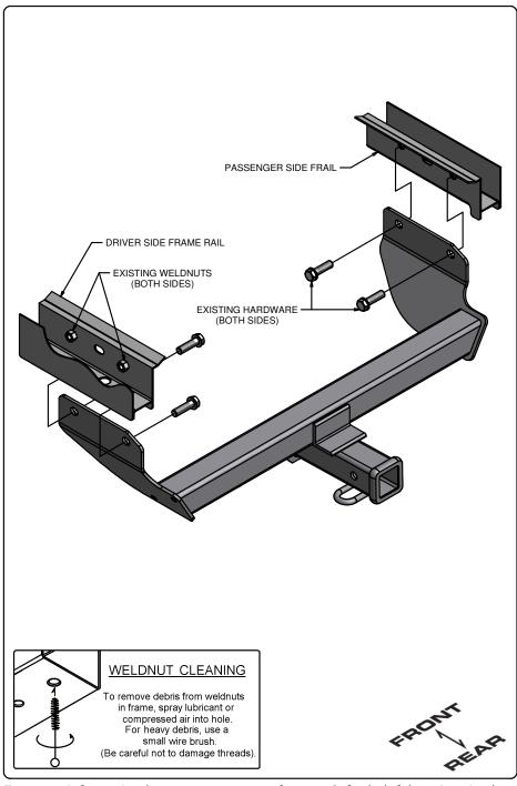
1. Remove (4) existing M14 bolts. These bolts will be used for hitch installation.
