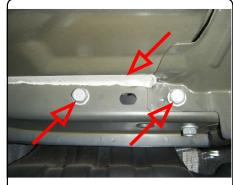
2. Raise hitch into position and reinstall (4) M14 bolts. Torque all M14 hardware to 126 ft-lbs.
