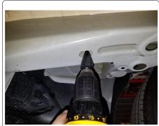
4. Fishwire (2) 7/16" carriage bolts and (2) CM-SP2 spacers through the access hole, located towards the front of the rail, into each frame rail.
