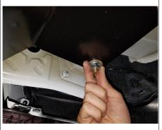
6. Torque all 7/16" hardware to 59 ft-lbs. Reinstall following Step 1 in reverse order.
