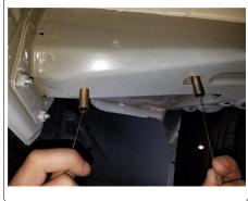
5. Raise hitch into position and loosely fasten (2) conical tooth washers and (2) 7/16" hex flange nuts on each side.
