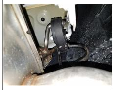
Locate and remove (3) bolts with a 10mm socket to remove the heat shield. Mark out a 9.25" x 10.50" section using masking tape and trim the heat shield. Reinstall heatshield. <u>NOTE</u>: If vehicle is dual exhaust remove (6) bolts and trim (2) heat shields. Reinstall after trim.
