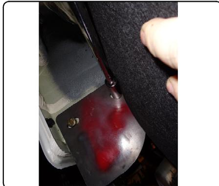
5. Raise exhaust back into position and secure to vehicle hanger.
