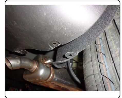
2. Lower exhaust by removing rubber exhaust hangers from hanger rods in (1) location on the passenger side.
