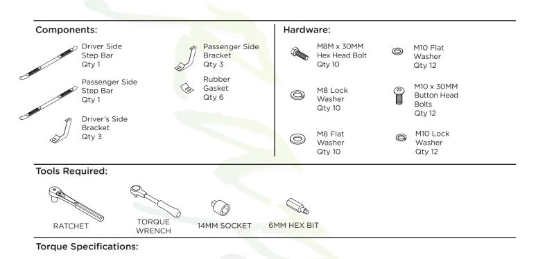
For Rocker Panel Mount Installations M8 through M12 bolts and nuts are set to 15-20 ft lbs.
