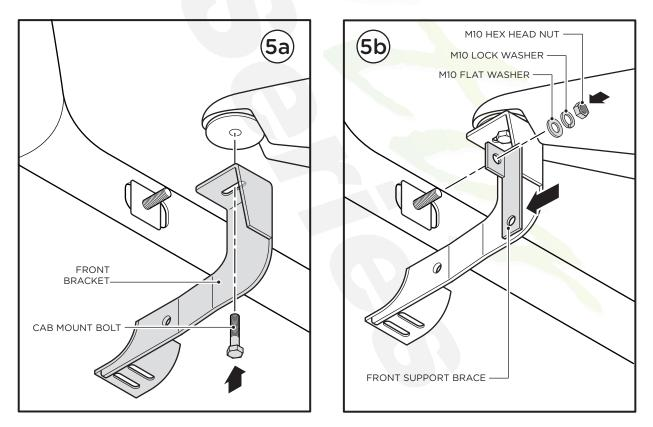
**6.** Fasten the Front Support Brace to the Front Bracket using one (1) M10 Lock Washer, two (2) M10 Flat Washers, one (1) M10 Hex Head Nut and one (1) M10 x 30MM Hex Head Bolt.
