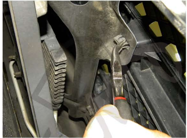
6. Unclip metal clips from rear of front grill
