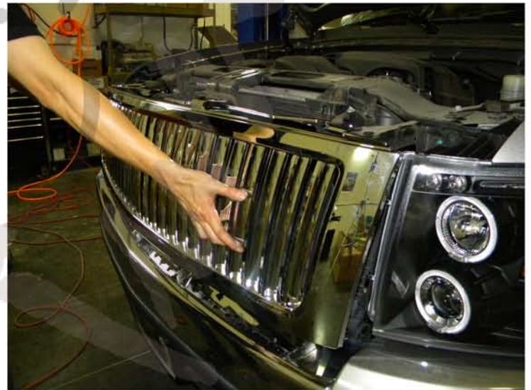
8. Place new grill in stock location
