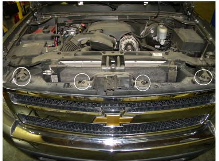
4. (4) 10mm bolts location
