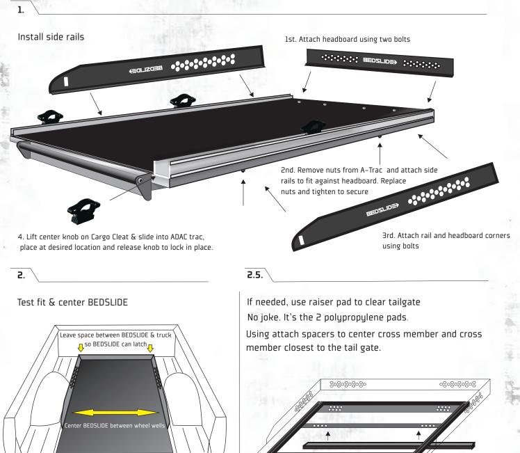
Make sure tailgate can close before drilling. Slowly slide BEDSLIDE out to make sure it clears tailgate in open position.
