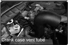
**17.** Drop the intake tube into the engine bay and connect the small end of the tube to the 4.00" straight hose on the turbo inlet. Also Connect the CCV tube to the port on the intake tube from figure 15
