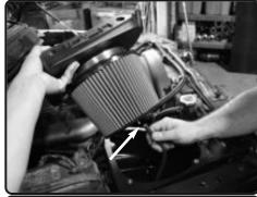
**12.** Connect the 3mm vacuum hose from figure 10 to the Filter Minder to the barbed fitting on top of the Injen filter.
