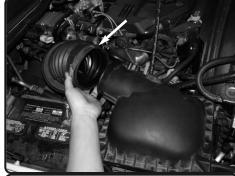
**4.** Loosen the clamp from the air duct to the air box assembly and then pull the air duct from the air box.
