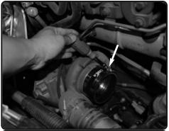
**16.** Place the 4.00" straight hose and two #64 clamps onto the turbo inlet and only secure the the clamp on the turbo side for now.
