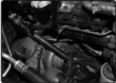
**15.** Connect the 17"-7mm vacuum hose to the crank case breather line. This vacuum line will connect to the Injen intake tube in figure 17
