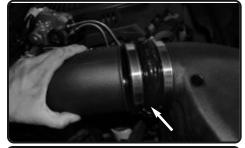
**18.** Push the upper part of the intake tube into the 4.50" hump hose on the intake plenum. Slide the hump hose towards the intake tube till it's centered. Adjust intake tube for best fitment and then secure all the clamps.
