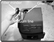
**3.** Place the grommet onto the drilled hole on top of the Injen air box. Connect the vacuum line to the filter minder then run the Filter minder into the grommet.
