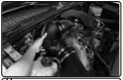
**11.** Insert the Injen intake tube into the 4.50" hump hose and the turbo end into the 4.25"-4.50" step hose. Once the intake is adjusted for best fitment, continue to secure the rest of the clamps
