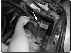
Remove the trim panel behind the passenger side headlight. Removing this panel will allow additional air into the intake system.
