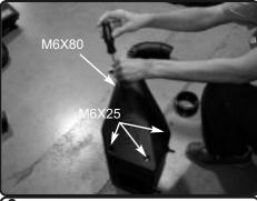
**6.** Place the three M6X25mm bolts and one M6X80mm into the plenum illustrated by the photo. Your Injen air box assembly is now complete.
