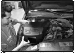
7. Lower the Injen air box assembly into the engine bay. Make sure the pegs under the injen air box goes into the facotry air box grommets located on the air box bracket.
