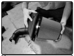
**4.** Place the filter onto the the Injen intake plenum and then secure the clamp.
