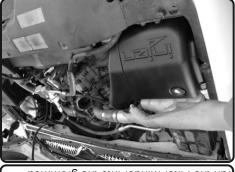
bracket. air box grommets located on the air box under the injen air box goes into the facotry into the engine bay. Make sure the pegs Lower the Injen air box assembly
