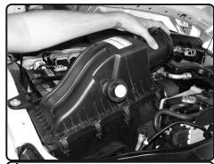
**4.** Lift the entire air box assembly out. Once air box is out. Remove the air duct from figure 3
