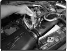
**16.** Connect the other end of the tube to the Injen air box plenum and push the 4.50" hump hose over. Adjust the intake system for best fitment and secure clamps.
