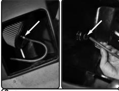
**9.** Connect the 3mm vacuum hose to the 1/8" fitting on the filter. Then connect the other end to the filterminder from figure 6.
