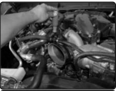
**12.** Place the 4.50" straight hose and two #72 clamps onto the turbo inlet. Only secure the clamp on the turbo inlet for now.
