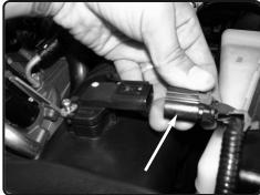
Disconnect the MAF sensor harness from the MAF sensor on the air box assembly.
