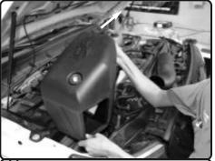
**11.** Drop the complete Injen airbox onto the mounting grommets from figure
