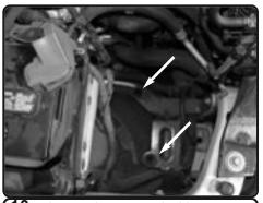
**10.** Locate the two stock airbox mounting grommets. The injen airbox will also use these two grommets to mount up.
