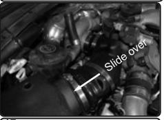
**17.** Push the 3.0" end of the Injen tube into the 3.0"-4.0" step hose on the turbo. Then slide the 4.5" hump hose over to the Injen air box side.
