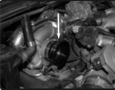
**15.** Place the 3.0"- 4.0" step hose with #64 and #48 clamps onto the turbo inlet. Secure only the clamp on the turbo side for now.
