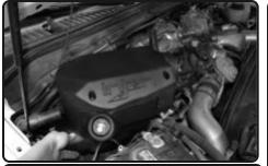
**13.** Drop the Injen air box assembly onto the three grommets from figure 12. Make sure the air box inlet inserts into the injen lower inlet. <u>Shifting the box left and down will help assist on securing the air box.</u> The air box will not move once in place
