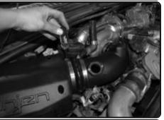
**18.** Once the Injen intake tube is in position, secure all the clamps
