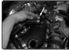
**19.** Use the supplied #16 clamp and secure the crank case vent tube to the port on top of the Injen intake tube.
