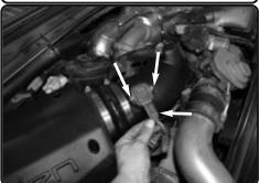
**20.** Use the supplied M4X10 bolts and secure the MAF sensor to the intake tube and then reconnect the MAF sensor harness
