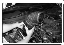
**5.** Loosen the clamp and the CCV line on the air duct connected to the turbocharger inlet and crank case breather line and then remove the entire air duct.
