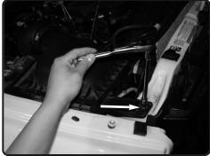
**3.** Remove the 13mm bolt from the air box assembly on the radiator support.
