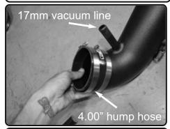
**17.** Place the 4.00" straight hose and two #64 clamps on to the end of the Injen intake tube and then connect the 17mm vacuum to the port on the intake tube.
