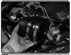
**20.** Place the 4.50" hump hose and two #72 clamps onto the top end of the intake tube.
