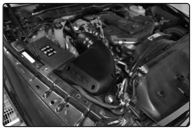
Congratulations! You have just completed the installation of this intake system. Periodically, check the alignment of the intake, normal wear and tear can cause nuts and bolts to come loose.
