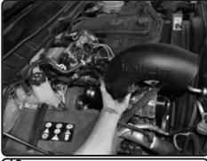
**18.** Attach the intake tube to the turbocharger and then connect the 17mm vacuum line to the CCV tube on the engine.
