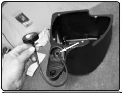
**13.** Install the grommet onto the air box bracket. connect the 3mm vacuum hose to the filter minder and then insert vacuum line and filter minder into the grommet.
