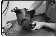
**11.** Firmly press the active door back onto the motor on the Injen air box. Make sure the active door is fully bottomed out. An "Active Air Door"" warning light may trigger if not properly installed.
