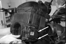
**6.** Firmly lift up on the entire air box assembly and remove it from the engine bay. Unscrew the active air duct motor assembly from the OE air box.
