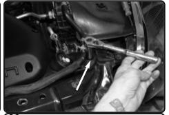
**23.** Use the M8X40 bolt to secure the air box bracket to the radiator support
