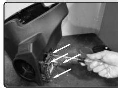
**12.** Re-use the 4 factory torx bolts and secure the motor to the Injen air box.
