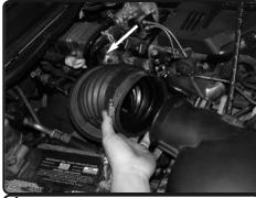
**4.** Loosen the clamp from the air duct to the air box assembly and then pull the air duct from the air box.
