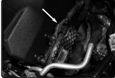
**22.** Re-connect the active door motor harness on the side of the air box.
