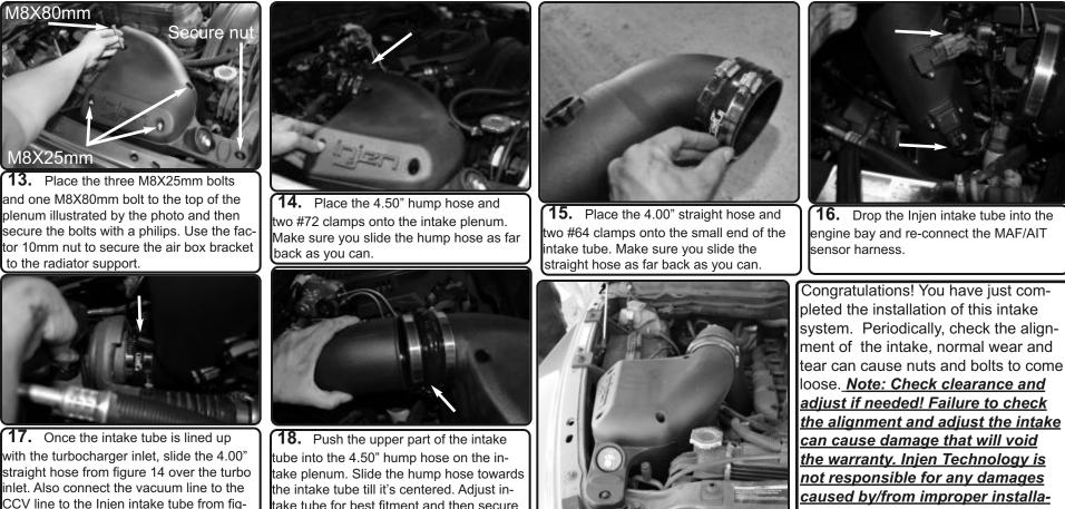
engine bay and re-connect the MAF/AIT sensor harness. Congratulations! You have just completed the installation of this intake system. Periodically, check the alignment of the intake, normal wear and
