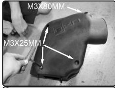
**8.** Place the three M6X25mm bolts and one M6X80mm into the plenum illustrated by the photo
