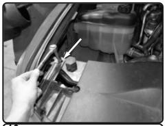
**10.** Use a 10mm socket/rachet to remove the 10mm bolt from the passengerside headlight.
