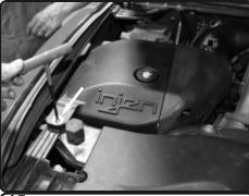
**15.** Place a M6X20mm button head bolt into the Injen air box mounting bracket. Secure the bolt to the chassis.
