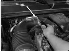
**3.** Loosen the clamp on the stock air box air duct to the turbo inlet.
