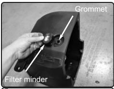
**5.** Place the grommet onto the drilled hole on top of the Injen air box. Push the Filter minder into the grommet.
