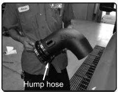
**13.** Place the 5.00" hump hose and two #80 clamps onto the big end of the lnjen intake tube
