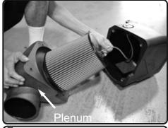
**7.** Place the filter onto the plenum and secure the clamp. Then connect the 3mm vacuum hose from figure 6 to the barbed fitting on the filter
