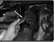
2. Disconnect the MAF sensor harness. Loosen two torx bits and remove MAF sensor from the stock air box assembly.
