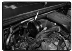
**9.** Place the 4.25X2.75" Straight hose and two #72 clamps on to the turbo inlet. Secure the clamp on the turbo inlet only for now
