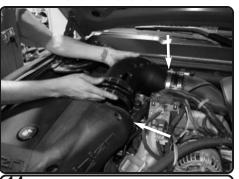
**14.** Place the small end of the Injen tube into the 4.125" straight hose on the turbo inlet and the other end into the Injen air box. Slide the 5.00" hump hose over the Injen air box
