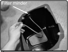
**6.** Connect the 16"- 3mm vacuum line to the filter minder
